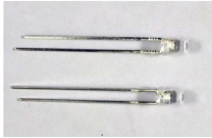
Figure 5 - PT19 Sensors – note the “Flag” side, short lead is the collector.
