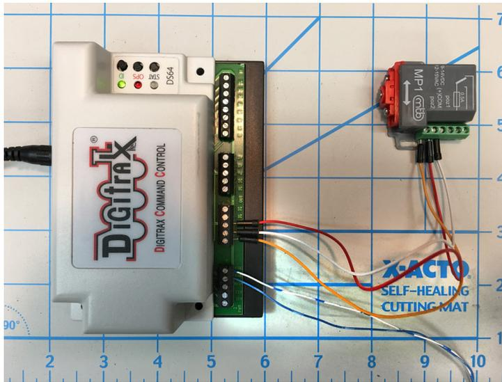
Figure 12 - MP1 with DS64 as the first device
