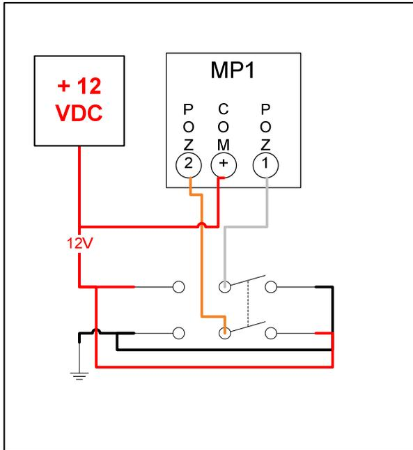
Figure 4 - DPDT Stall Motor installation Adapted for MP1
