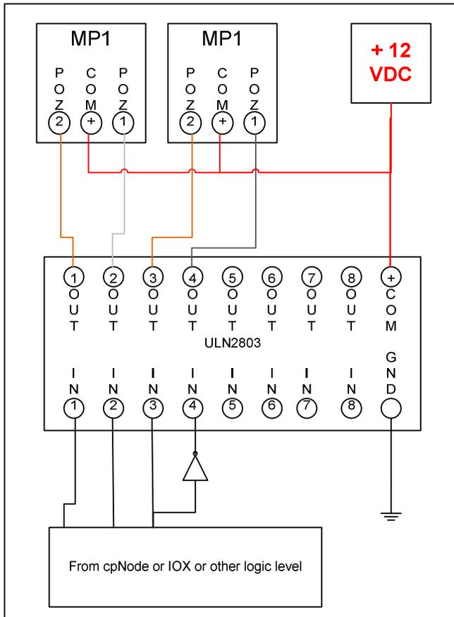
Figure 8 - ULN2803 drivers - Equivalent to one half of a CSNK
