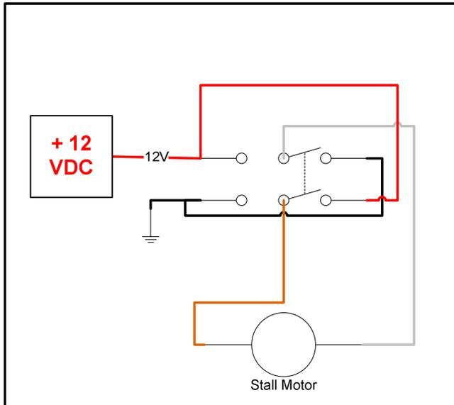
Figure 3 - Stall Motor Control with DPDT Switch
