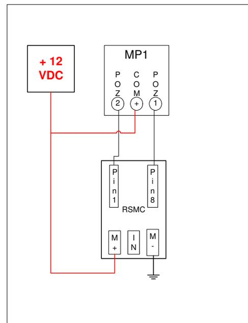
Figure 6 - RSMC Connections
