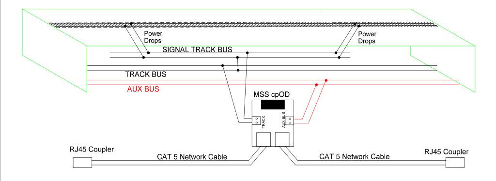
Using the MSS cpOD Crossover Board to simplify adding signal detection to a Free-mo module. The Crossover wiring is built-in to the Board!
