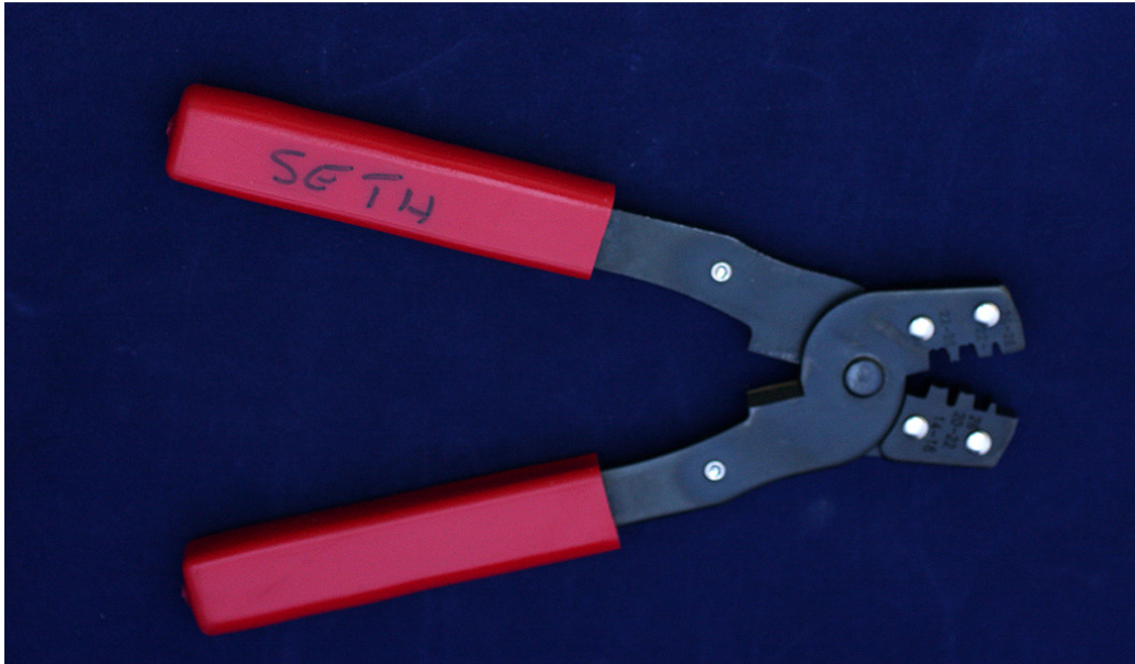
Figure 2 – Crimper, usually described as for RS232 pins
