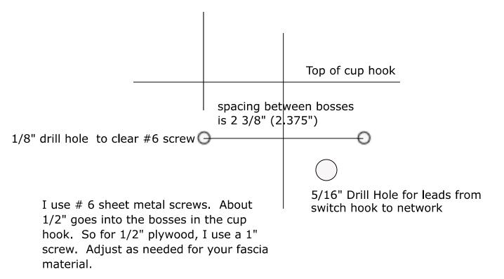
NOTE: paper is not dimensionally stable and some printers and copiers shrink or expand when printing so check dimensions before drilling!
