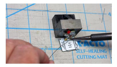
11. Trim any loose bits of circuit board that stick out with an old (not your good one) rail nipper and dress with a file as required.
