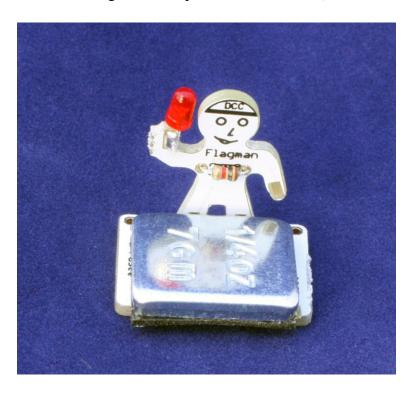
13. Place the large gold pads across the rails to light the red lantern. Not only can you flag on a dark railroad, but the Flagman draws about 10mA so it will force detection on a railroad using current detection. The Flagman also makes a handy tester for track voltage!
