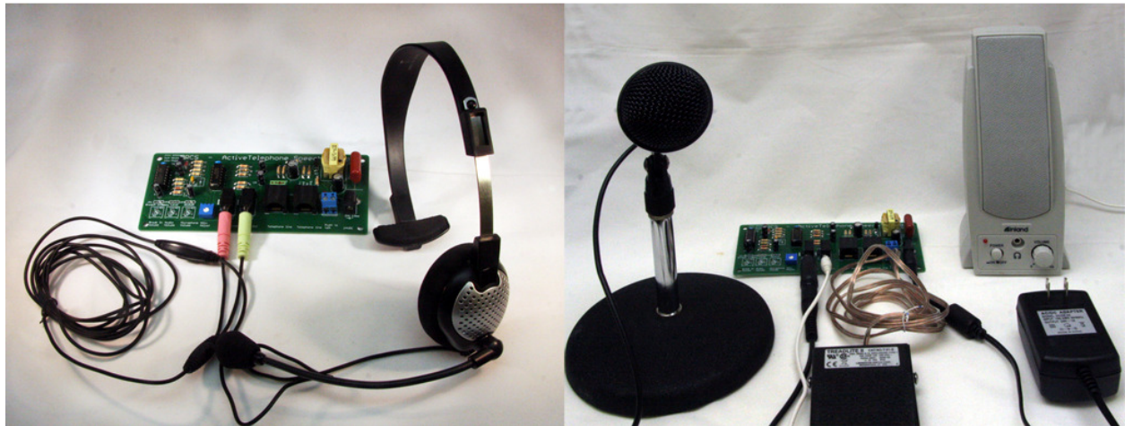
Figure 4 – Dispatcher/Operator Board with Headset and Mic/Speaker/Foot Pedal
