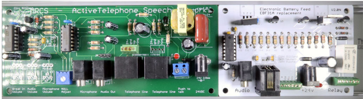
Figure 3 – Dispatcher/Operator and EBF31A boards in DINRail
