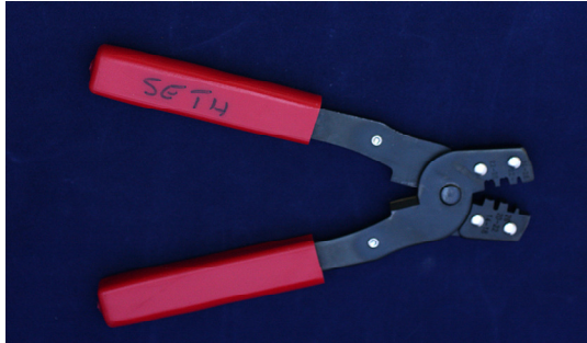
Figure 4 - Crimper for Spade Lugs - often called an RS232 crimper
