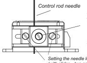
Needle mount and height adjustment – by moving axially the needle with the screw loosened (2 grooves for needles of different sizes)
