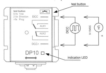
For the purposes of switch function testing, a DC power supply of 9-16V, with marked polarity, can also be used. Only for functional test, by buton.
