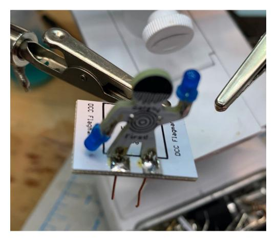
Clip the wires on the bottom of the base, add the weight (see placement box on the base). Now test!
