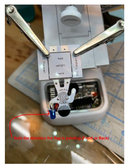
Clip the leads of the Blue LED to about ¼" and straddle the board, solder to the front and back (shown). Note direction of the flag, you'll do the other arm opposite. When you're done with the right arm, snap the base off so you can easily get to the left arm.
