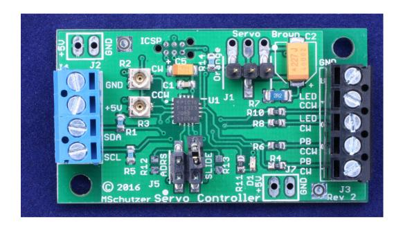
Our compact Servo Controller is another Mark Schutzer design. It can drive one servo, such as the popular SG90. The controller provides all of the electronics required to control one servo (except 5VDC power). Servos are ideal for applications where precise positioning of the end of travel is required and their small size and the variety of linkage hardware for them (from the R/C community) makes them well suited for installations in tight spaces. The Servo Controller features:
