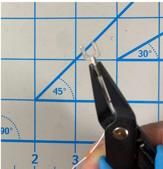
Figure 7- Grab the barrel of the lug with spiking pliers (use the groove to align the lug)
