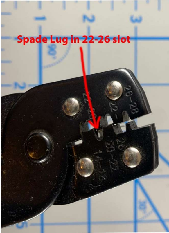
Figure 4 - Insert tail or "butt" of lug into the 22-26 Ga Slot, note the open side of the butt goes into the slot
