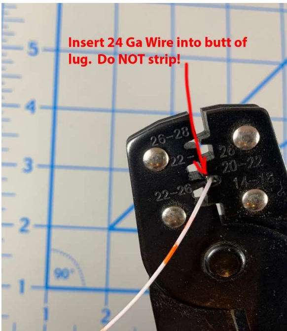
Figure 5 - Insert 22-26 wire into the butt of the lug, DO NOT STRIP!
