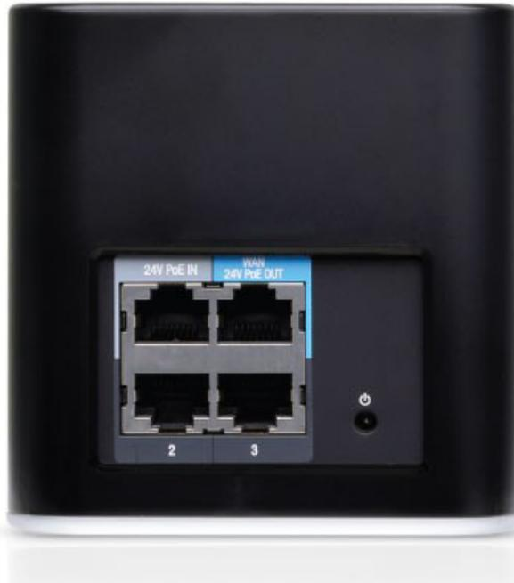
Connect a network (Ethernet) cable (supplied by user) from the AirCube WiFi Adapter port labeled “24v Poe IN” to your Cable Modem or Home Router. Plug in the AC power adapter.
