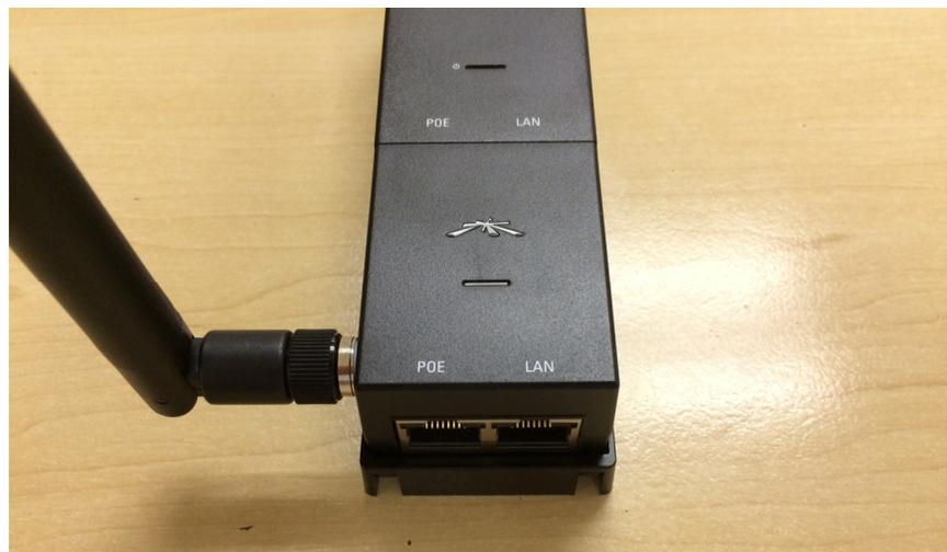
Connect a network (Ethernet) cable (supplied by user) from the AirGateway WiFi Adapter port labeled "LAN" to your Cable Modem or Home Router. Plug in the AC power cord.
