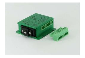
The MP5 is a slightly larger package than an MP1with a DPDT contact (one side for frog power switching and the other for position feedback or lighting a LED to show position (You can't use the series bi-polar LED trick with MP Motors). MP5 features a removable screw-less connector, 2 or 3 wire control, and 3,6,9, and 12 mm throw adjustments. The removable connector sticks out about 10mm (~0.5"). Size including mounting ears and connector: 1.7" x 2.5" x 0.76" (43mm x 63.5mm x 19.27mm)
