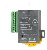
The MP10 is similar to the MP4 except that it has the mechanical footprint of a Tortoise by Circuitron (tm) motor. However the MP10 is only 20mm (~.75") high as opposed to the Tortoise's 83mm. MP10 uses the same removable screw terminal connector as the MP4, 2 or 3 wire control, and 3,6,9, and 12 mm throw adjustments. Size including mounting ears and connector: 2.3" x 2.2" x 0.8" (58 mm x 55 mm x 20 mm)
